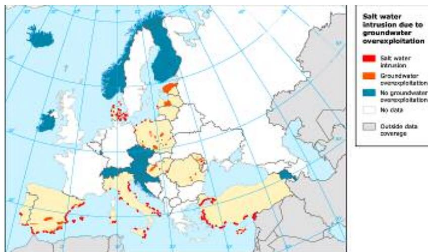
**Fig. 5** - Salt water intrusion due to groundwater intensive exploitation (copyright EEA, Copenhagen, 2005)
